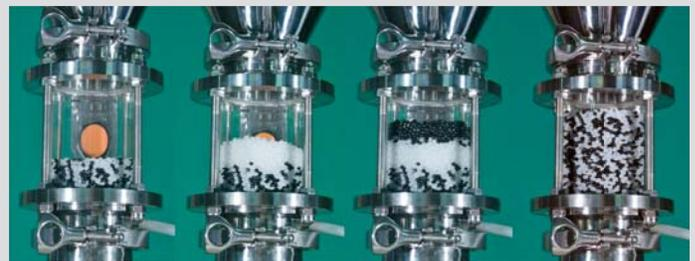
The SMB blender uses Turbo Blend technology to re blend the material once it arrives at the feed throat. In most cases the material arrives pre blended as it is fed onto the conveying stream in the correct proportion. In some cases with low percentages of color it is necessary to re blend the material. The SMB Blender starve feeds each shot so there is no place for material to accumulate and separate.
